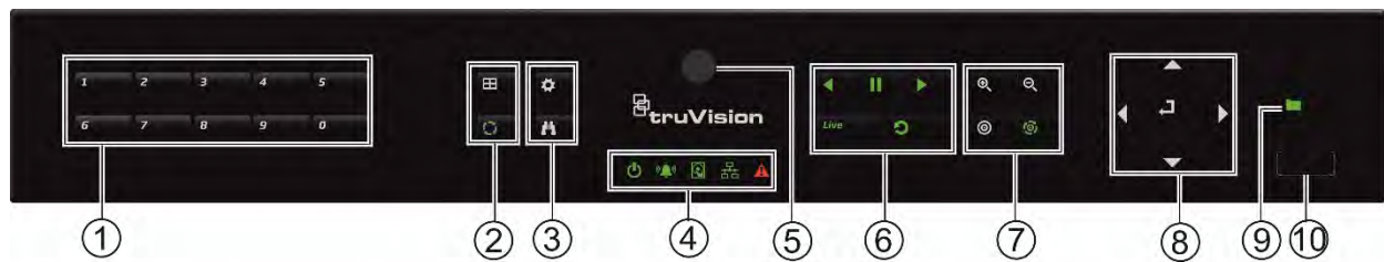
Figure 4: TVR 16 front panel
